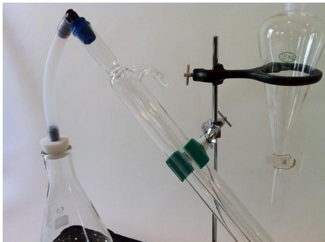
Next, connect the longer ¼ inch PVC tube from the water faucet hook-up or water pump to the bottom of the condenser and then another tube from the top of the condenser condenser back to the sink or draining location.
